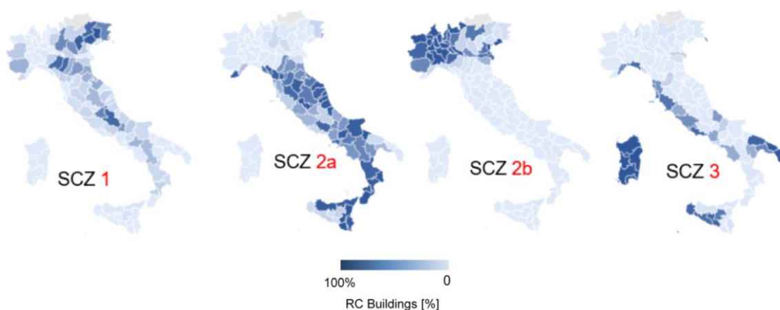
Figure 40. Distribution of Italian RC residential buildings in each SCZ by Italian province, according to local values of PGA and HDD (Level 2 – Detailed analysis)
