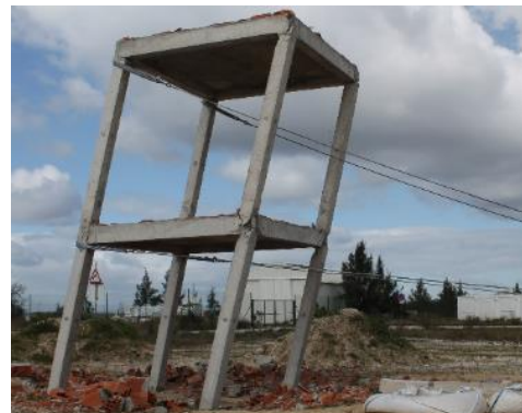
Full scale 3D frame structure under monotonic pushover
