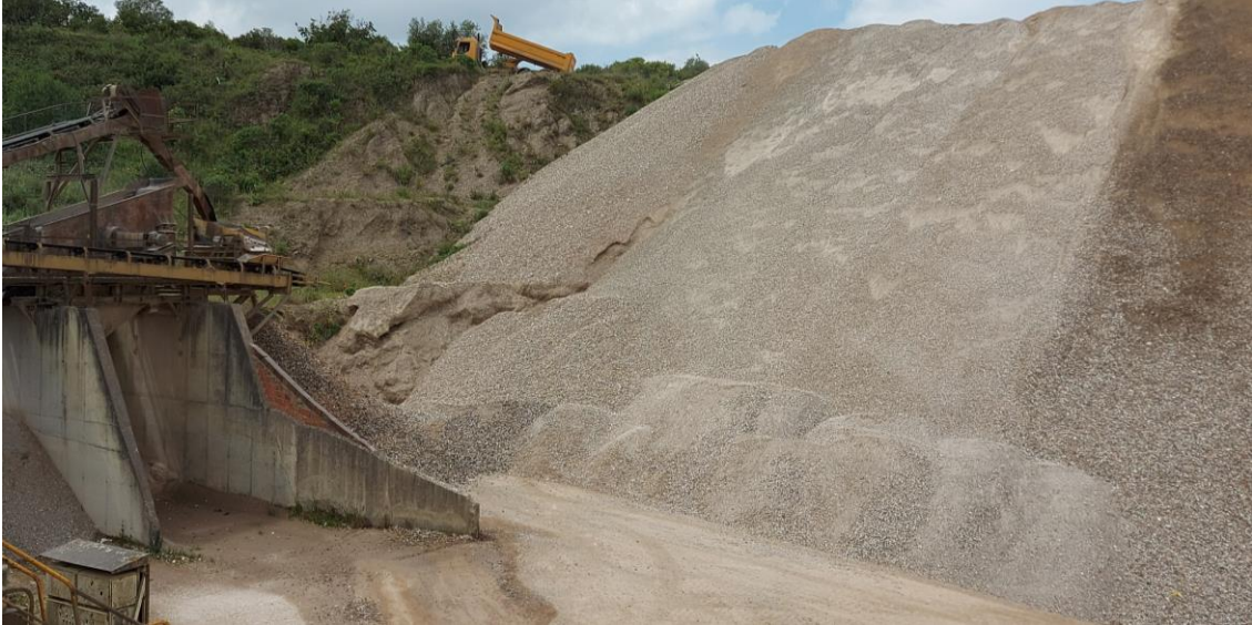
Figure 5. Treated waste processed into recycled aggregates stored at a CDW management facility indefinitely
