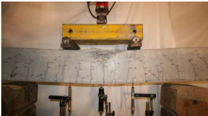
Beam tested for bending
