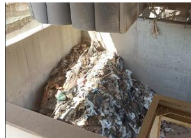
Light materials removed by air sifter
