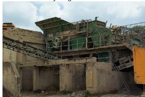
Jaw crusher with preliminary screen for removal of smaller particles
