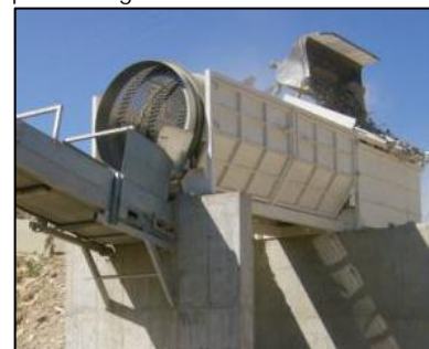
Trommel for size classification of RA for road construction and other unbound uses
