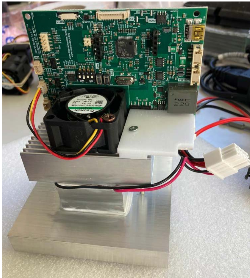
Figure 4. CO 2 sensor with temperature controlled elements and expansion shield (Expansion Shield 2)
