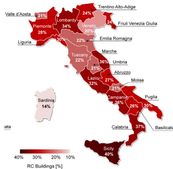
Figure 9. Geographical distribution of Italian RC residential buildings at regional level - Percentage of RC buildings over the total number of buildings in each region
