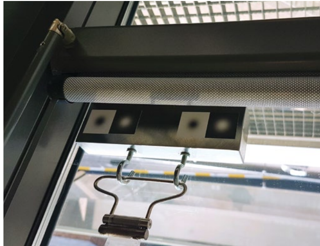
Figure 14: Peel test for assessing the behaviour of the adhesive in an ASF
