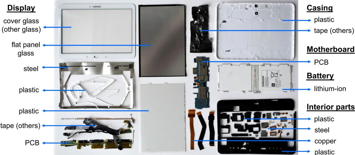
Figure 55: Example of product disassembly for a tablet (Samsung Galaxy Tab 4 SM-T530, 2014), illustrating the main components (Babbitt et al., 2020).
