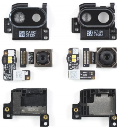
Figure 86: modular components of the Fairphone 3 smartphone.
