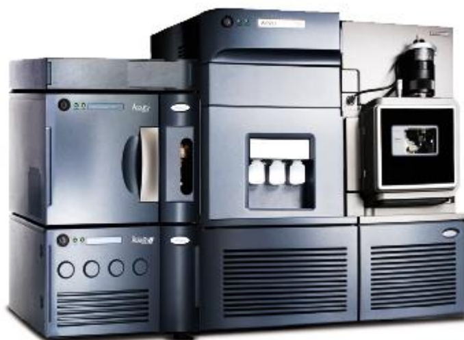
Figure 16. Acquity UPLC - Xevo TQ-S MS. Source: Degryse et al., 2017
