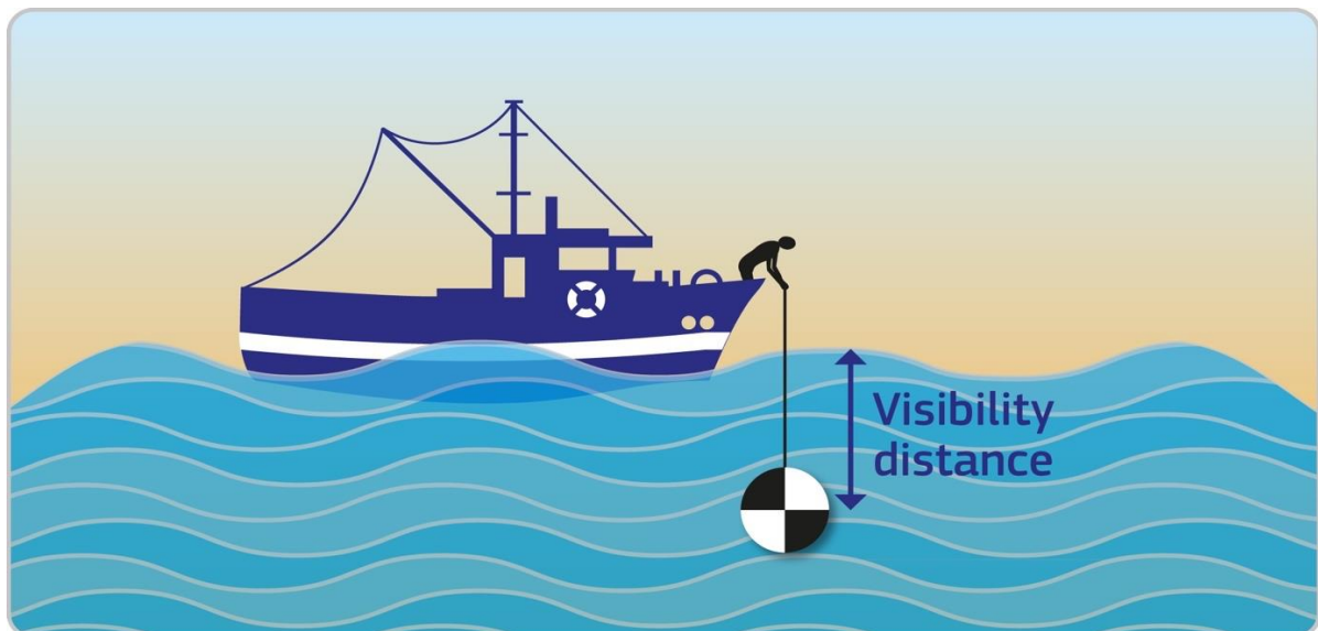
Figure 2. Measurement of water transparency using a Secchi disk. The Secchi disk is lowered by the operator into the water and the depth at which the disk is barely no longer visible (termed “Secchi depth”) is recorded.
