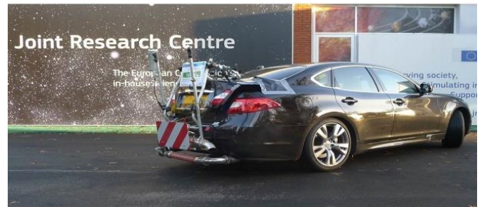
Figure 1 – Light-duty vehicle equipped with a PEMS, ready to perform a RDE test
