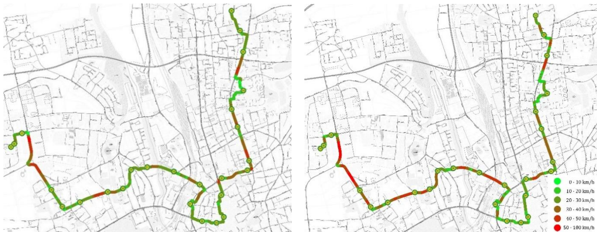
Figure 76. Analyzed bus line with the color indicating the vehicle speed. Left: Speed profile from SUMO simulation. Right: Speed profile from the actual bus
