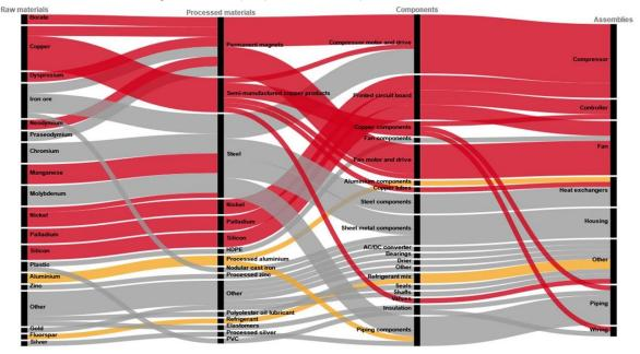
Figure 33. Heat pumps materials, components and assemblies
