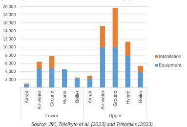
Figure 9. Typical up-front costs for individual heating systems in the EU (euros)
