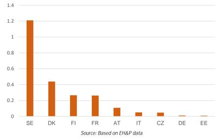
Figure 7. Installed capacity of large heat pumps in district heating and cooling networks by Member State, 2021 (GW)
