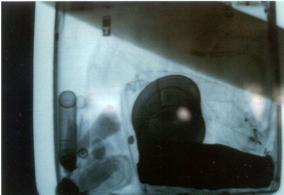
Figure 5: X-ray photo of the suitcase containing the can of plutonium-uranium powder and the piece of lithium metal
