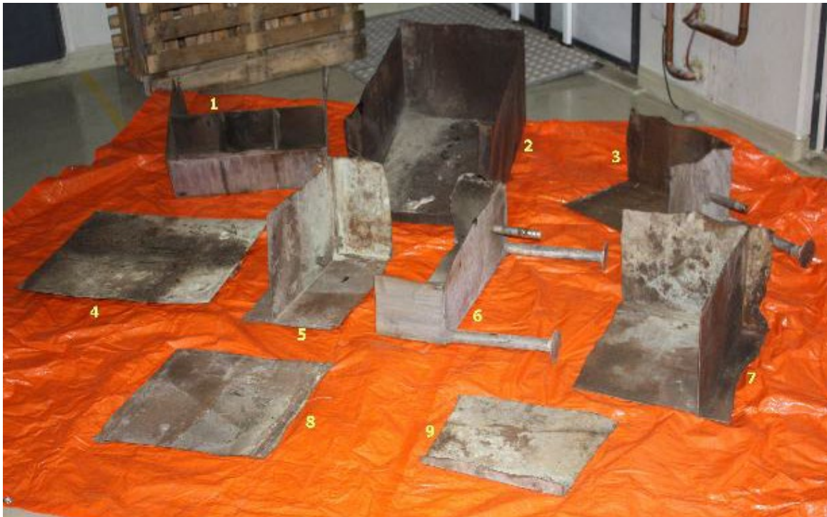
Figure 6: The objects found at a scrap metal yard contaminated with uranium
