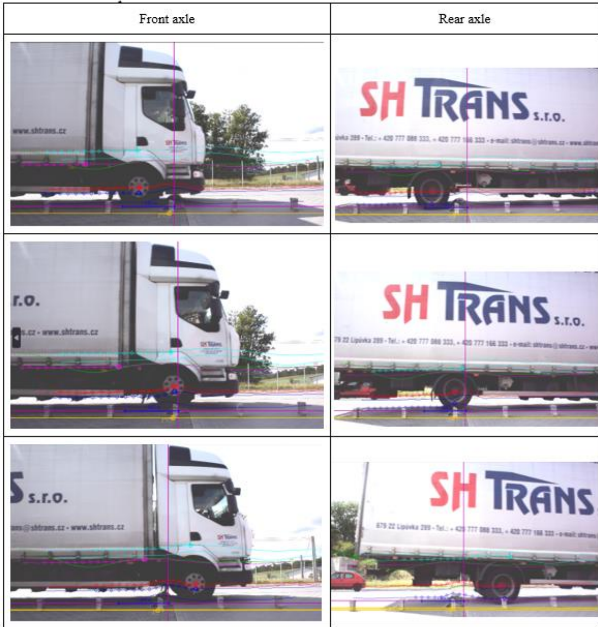
Figure 60: Curb test experiment – 16 km/h
