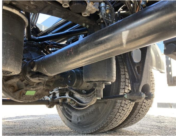
Figure2: Rear axle and wheel suspension
