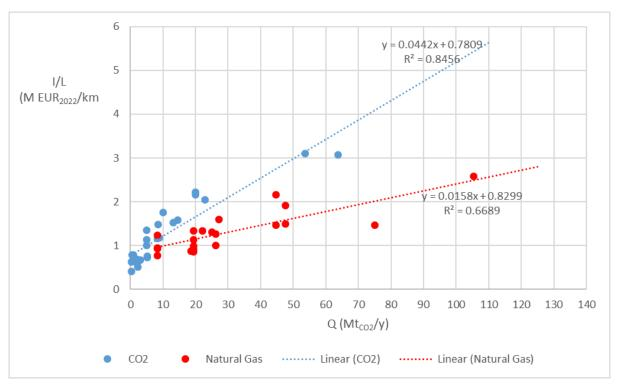
Figure 5. Estimation of onshore pipeline transport costs (CO<sub>2</sub> – blue, Natural gas – red)
