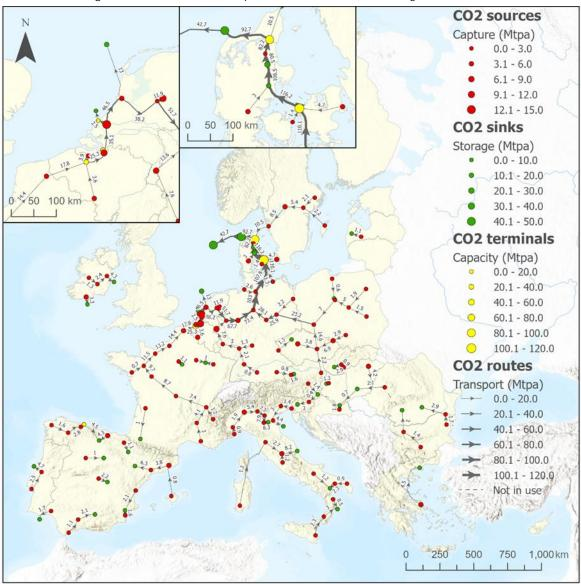
Figure 1. Potential CO<sub>2</sub> transport network in 2050 according to scenario C1
