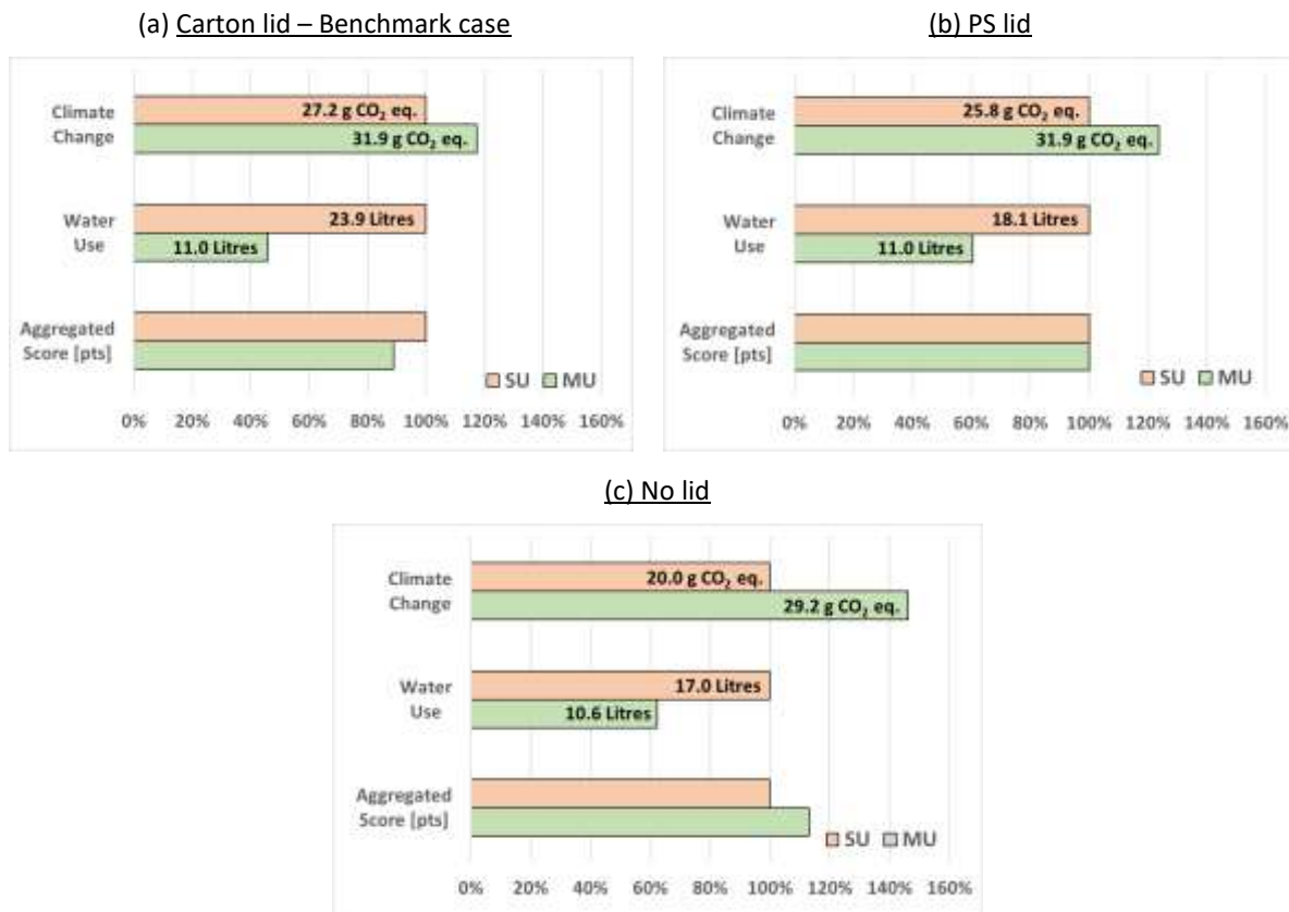
Figure 12. Results of the specific analysis of lid types for the Single Use (SU) and Multiple Use (MU) packaging products. The graphs illustrate the results for (a) SU packaging product including a carton lid with low-density polyethylene (LDPE) lining and (b) SU packaging including a polystyrene (PS) lid. The bottom graph (c) illustrates the results where both packaging products do not include any lid. SU impacts are set to 100 % for each impact category considered.
