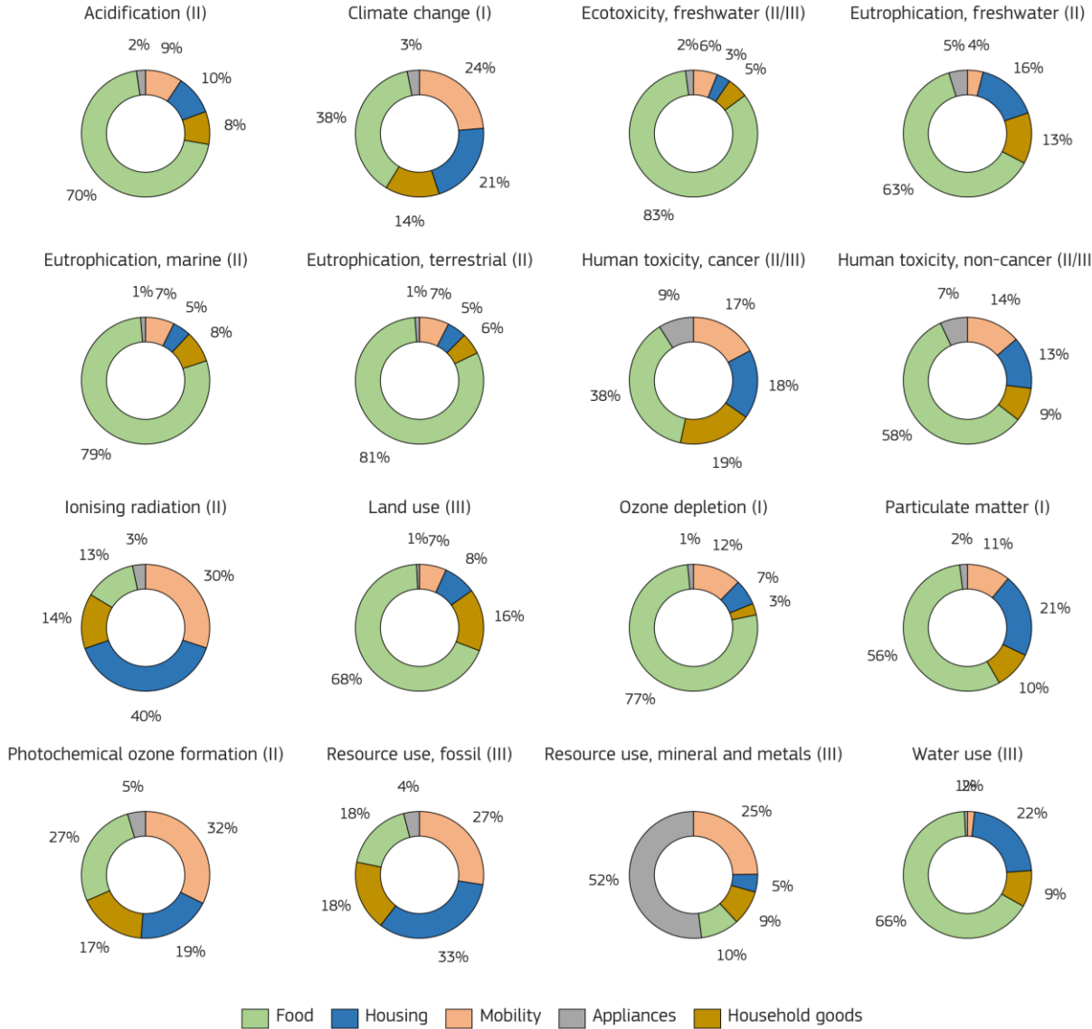
Figure 14. Environmental impacts contribution of the different areas of consumption for EU-27 expressed as in the 16 impact categories of the environmental footprint (2022).
