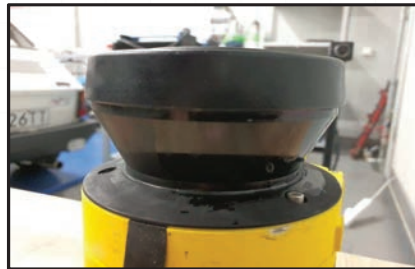
Fig. 8. Condensation of water vapor on the sensor's surface
