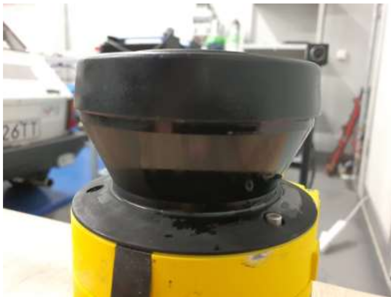
Figure 8. Scanner frosting (layer of condensed water steam prevents measurement)
