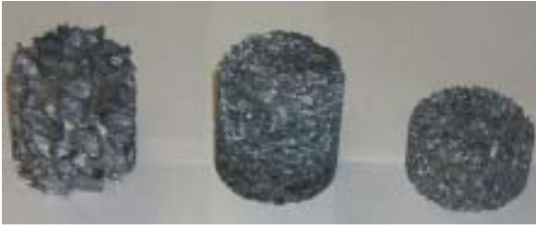
Aluminium foam specimens of very low and of higher density (cylinders of 50mm diameter and 50mm and 25mm height).
