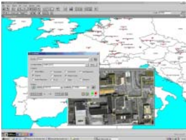
Screen dump of NUMAS showing the distribution of nuclear locations, together with the main attribute dialog box of a selected site and its VHR satellite image
