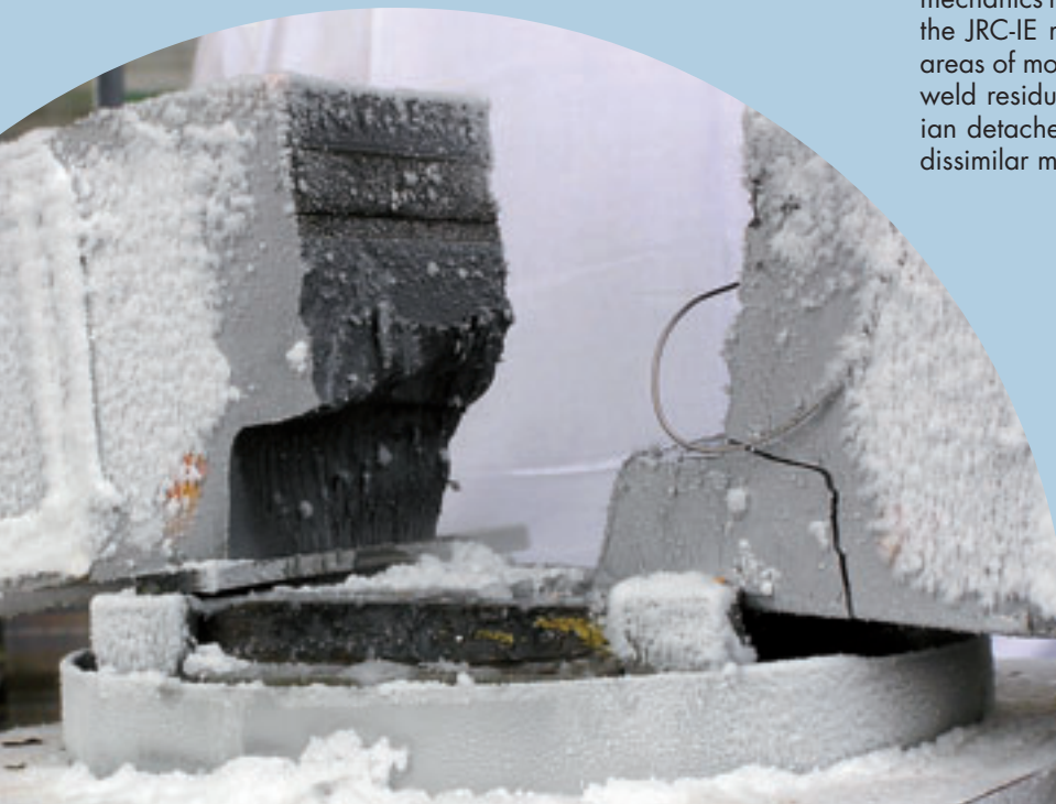
Fig. 5 - Tests on beams with simulated sub-surface flaws.
