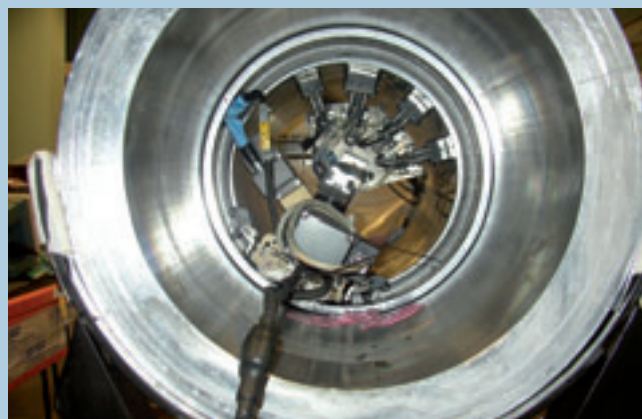
Fig. 7 - Inspection by ultrasonics from the inside of the piping segment containing two dissimilar metal welds. Unknown defect must be detected and sized within \pm 3 mm by the eight participating teams.
