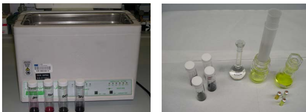
Picture 2: Various steps of method EN 14362: a) reduction; b) liquid-liquid extraction using diatomaceous earth column.
