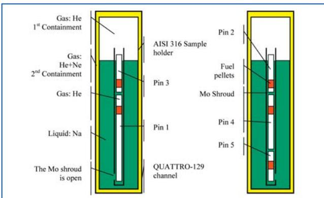
Figure 19 - Schematic view of the irradiation experiment. HELIOS1 on the left (pins 1 and 3), HELIOS2 on the right (pins 2, 4, and 5)
