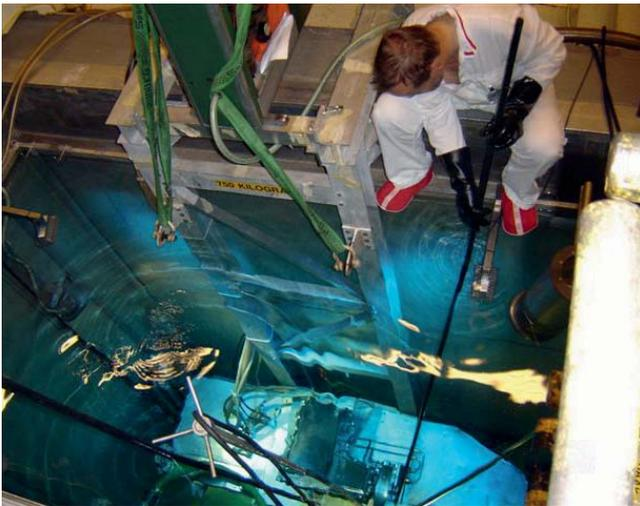
Figure 5 - Handling of the US owned test elements in the HFR pool
