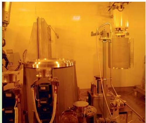
Figure 8 - The basket holding HEU elements is ready to be loaded into a canister in the hot cell at COVRA
