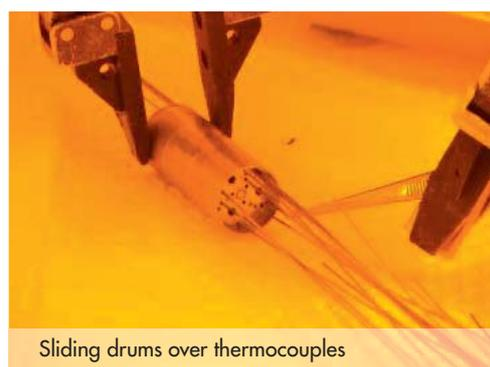
Sliding drums over thermocouples
