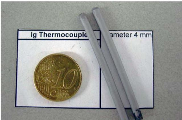
Figure 11 - Ig-type thermocouples tested (thermocoax)
