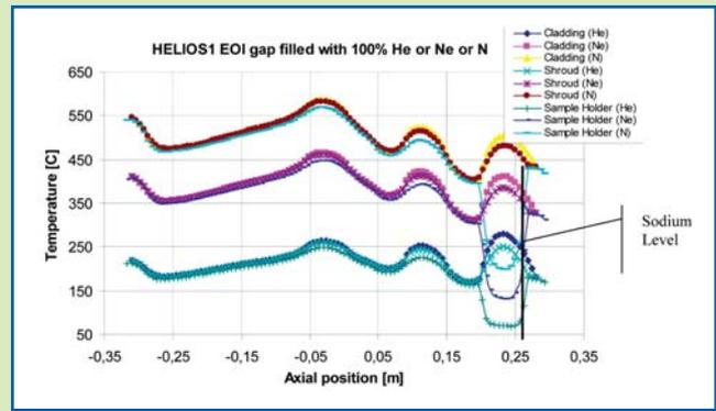
Figure 21 - Axial temperature profile of HELIOS1 at EOI, when the gas gap between the sample holder and the QUATTRO channel is filled with 100% Helium, Neon or Nitrogen
