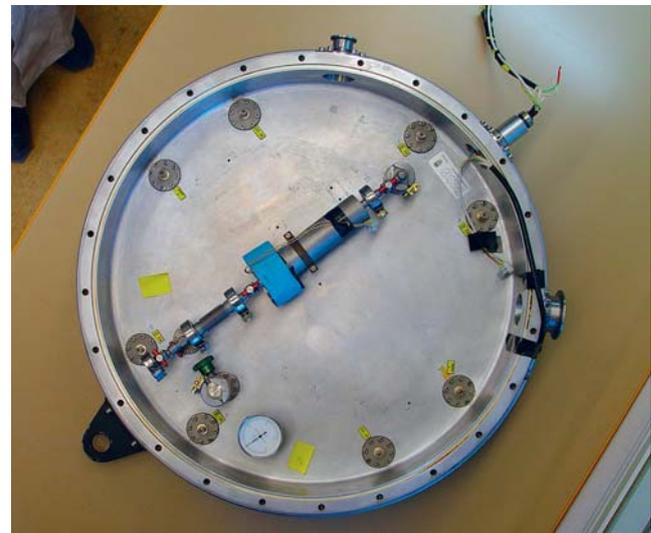
Figure 28 - SANS area detector during repair in JRC laboratory
