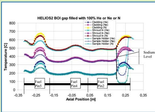
Figure 22 - Axial temperature profile of HELIOS2 at BOI, when the gas gap between the sample holder and the QUATTRO channel is filled with 100% Helium, Neon or Nitrogen
