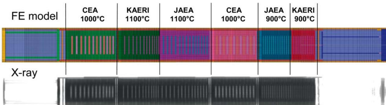
Figure 15 - Comparison between the Finite Element Design model, and the X-ray of the assembled experiment, showing that the assembled experiment is in excellent agreement with the thermo-mechanical design model.
