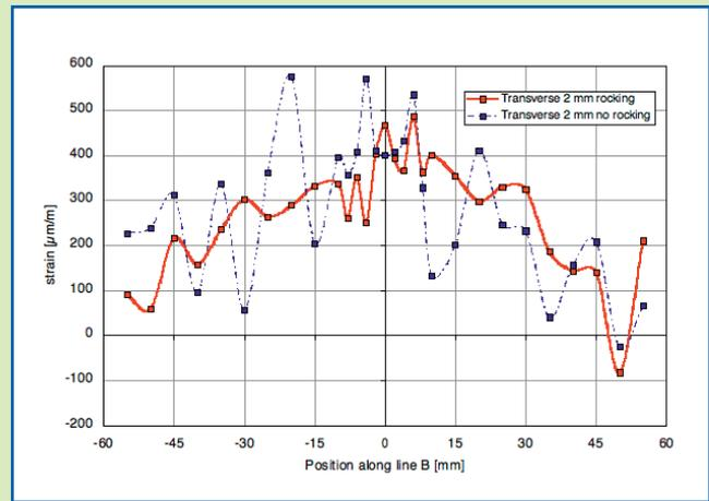
Figure 27 - Impact of measurement procedure in neutron diffraction; specimen "rocking" reduced the scatter in a data set obtained from a coarse grained welded steel plate
