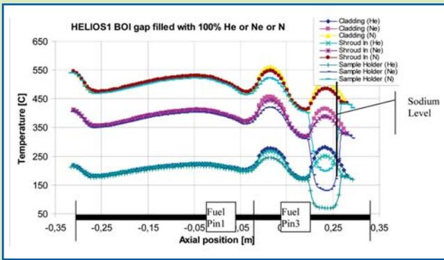
Figure 20 - Axial temperature profile of HELIOS1 at BOI, when the gas gap between the sample holder and the QUATTRO channel is filled with 100% Helium, Neon or Nitrogen
