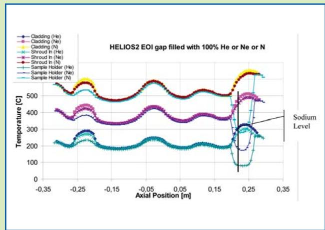
Figure 23 - Axial temperature profile of HELIOS2 at EOI, when the gas gap between the sample holder and the QUATTRO channel is filled with 100% Helium, Neon or Nitrogen
