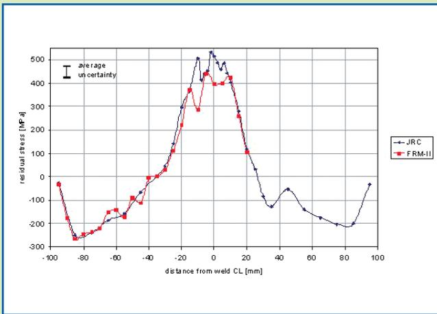
Figure 26 - NET TG2 Auxiliary specimen: welding longitudinal stresses measured at the HFR and at FRM-II, Germany
