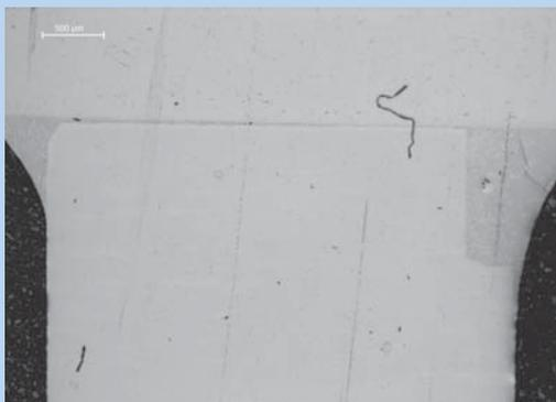
Brazing test on Ig-type thermocouples sheath
