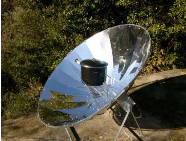
The K14 solar cooker fitted with the SUM.
