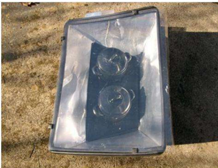
Top view of the SunStove solar box cooker produced in South Africa, fitted with two original pots and the SUM baseplate. The sensor cable (top), connects the base plate sensor with the SUM. Ambient temperature and irradiance sensors are integrated in the SUM housing.
