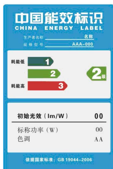
Figure 1 Energy Efficiency Label for Auto-Ballasting Fluorescent Lamp
