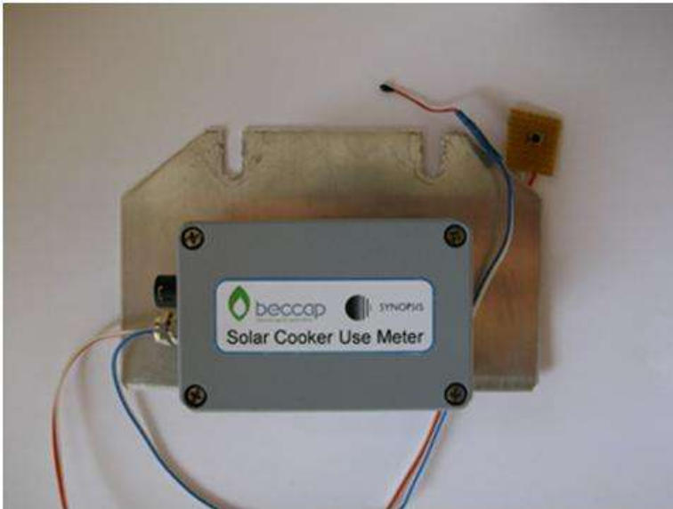
The K14 SUM with its external sensors for pot temperature, ambient and irradiance.
