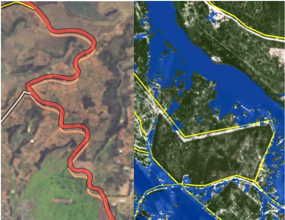
Figure 8 – Inconsistency between roads in thematic features and roads in the underlying image
