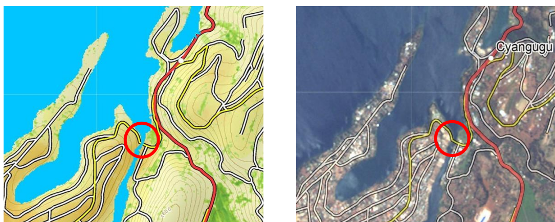
Figure 13- Example of topological inconsistency
