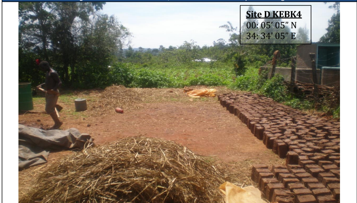
Figure 72: Detail site KEBK4, dried raw bricks ready for baking
