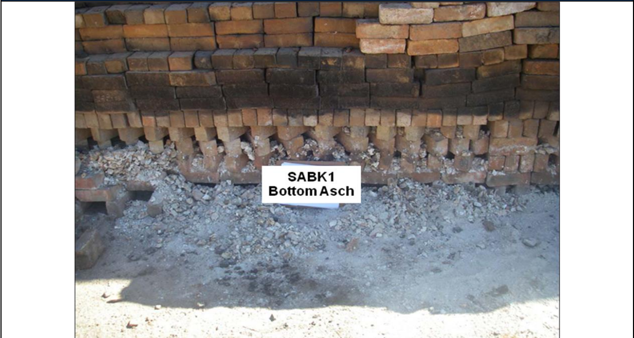
Figure 38: Detail SABK1, fired clamp kiln with bottom ash
