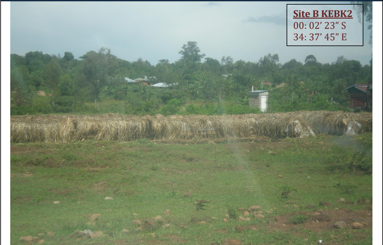
Figure 65: Detail KEBK2, drying of raw bricks (covered with grass)
