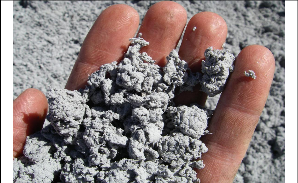
Figure 45: Detail SABK2, brick ingredient "fluff" (waste paper pulp)
