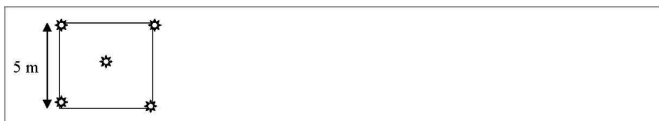
Figure 1: Scheme for the preparation of a composite sample made up from five individual samples
