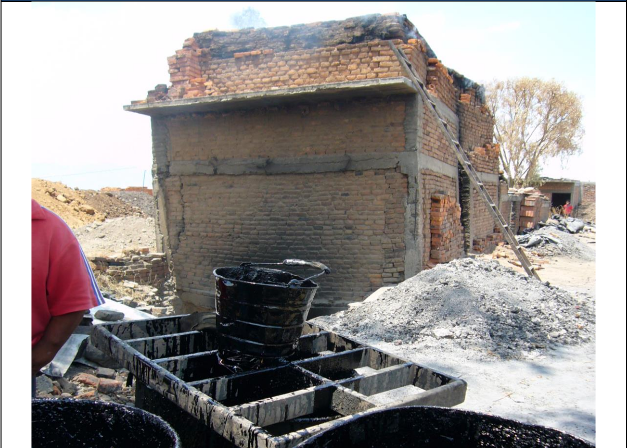
Figure 23: Detail Abasolo, Combustóleo and waste fired stationary kiln ( Brickash 2)
