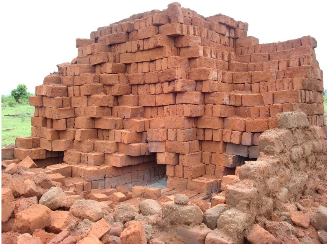
Partially dismantled kiln after the process Ash can be seen in the fire chambers
