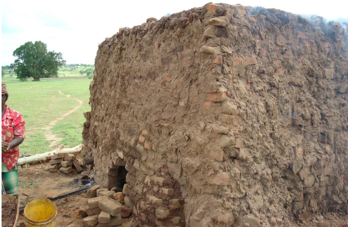
Baked brick covers the outside of the clamp, with mud used to seal the holes between
