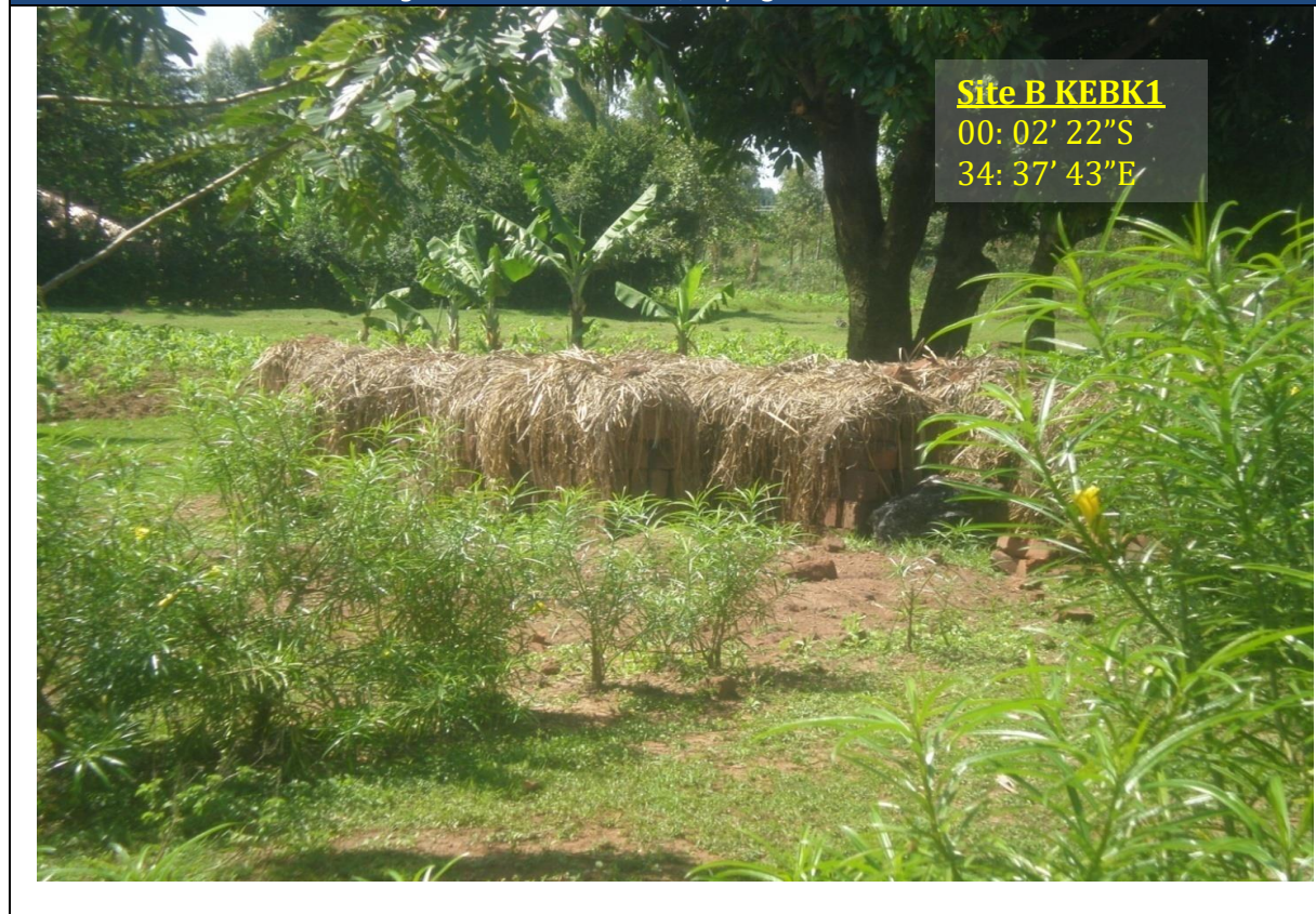
Figure 64: Detail KEBK1, drying of raw bricks
