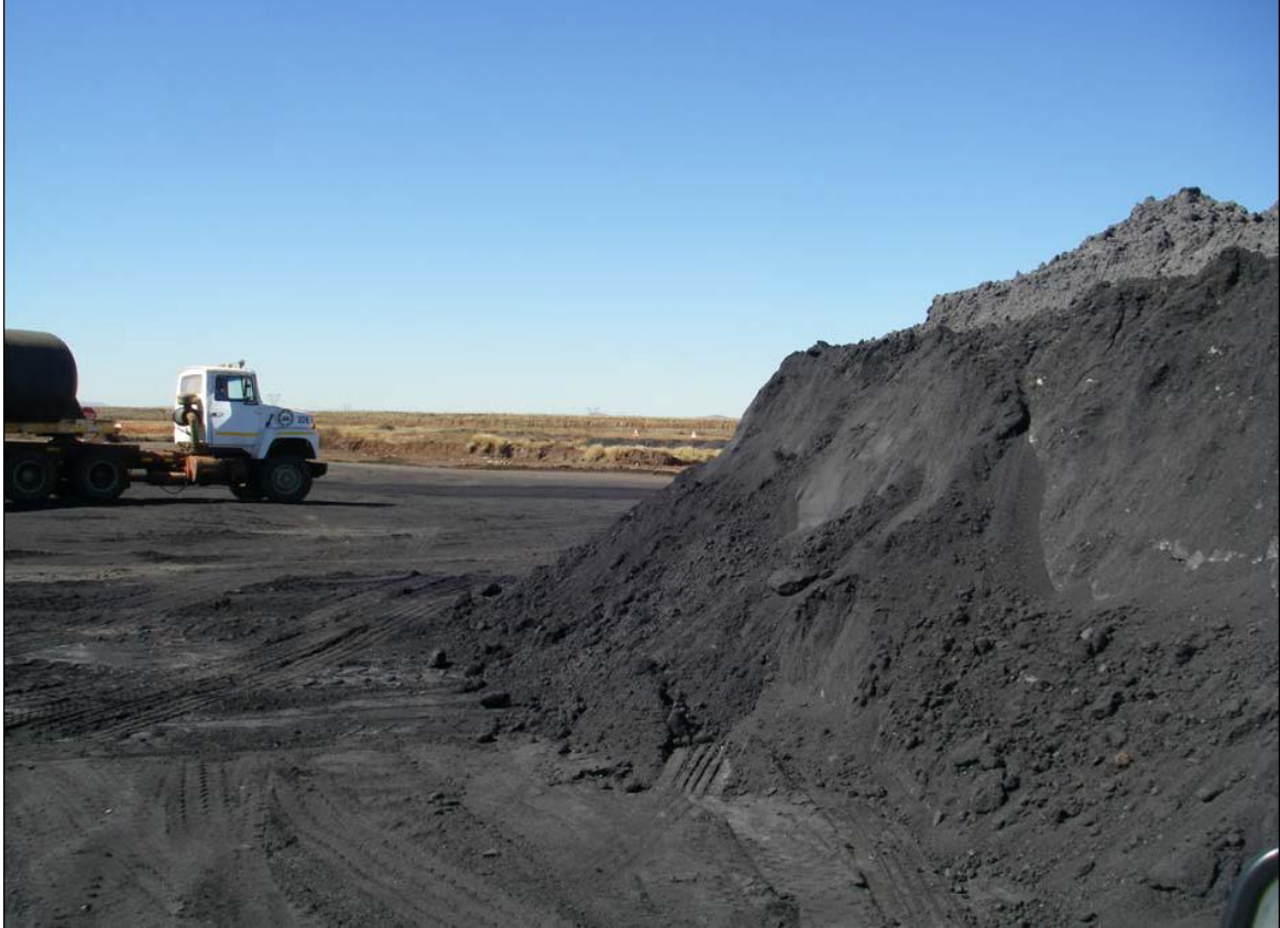
Figure 46: Detail SABK2, brick ingredient “duff” (fine coal)
