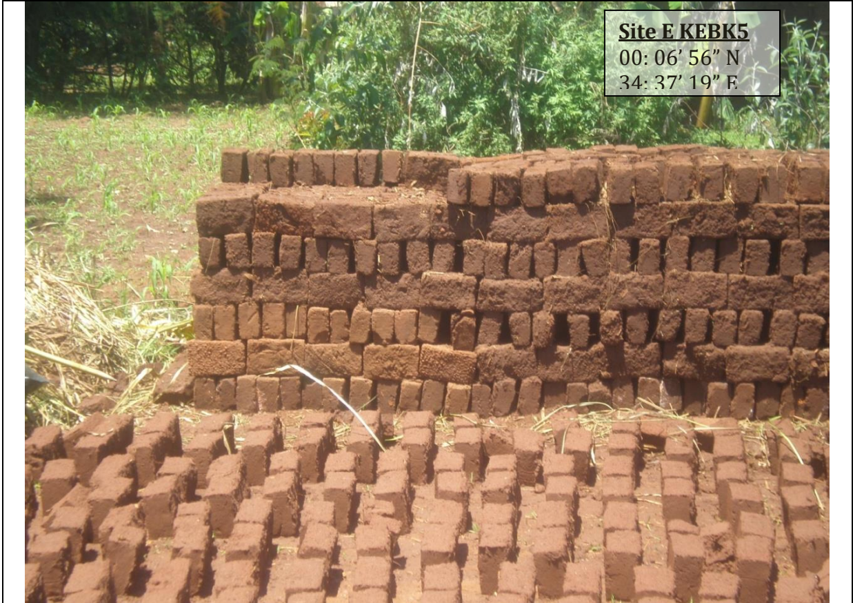
Figure 74: Detail site KEBK5, dried raw bricks prior to baking
