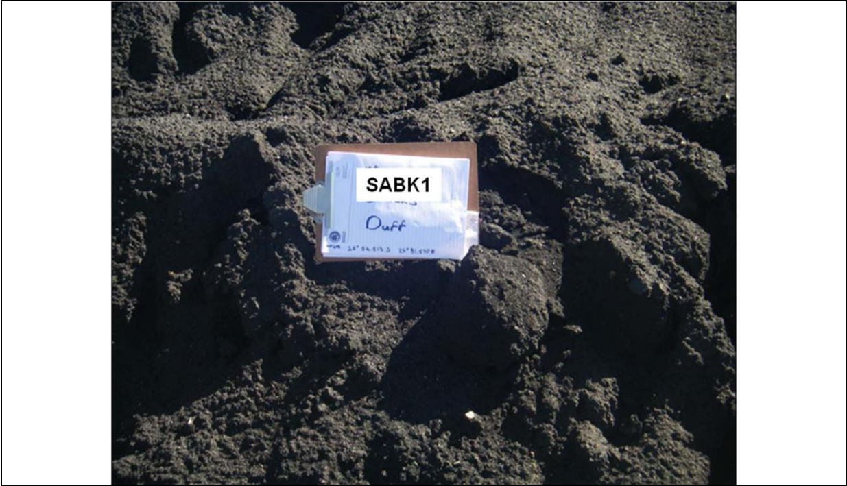
Figure 39: Detail SABK1, brick ingredient "duff" (fine coal)
