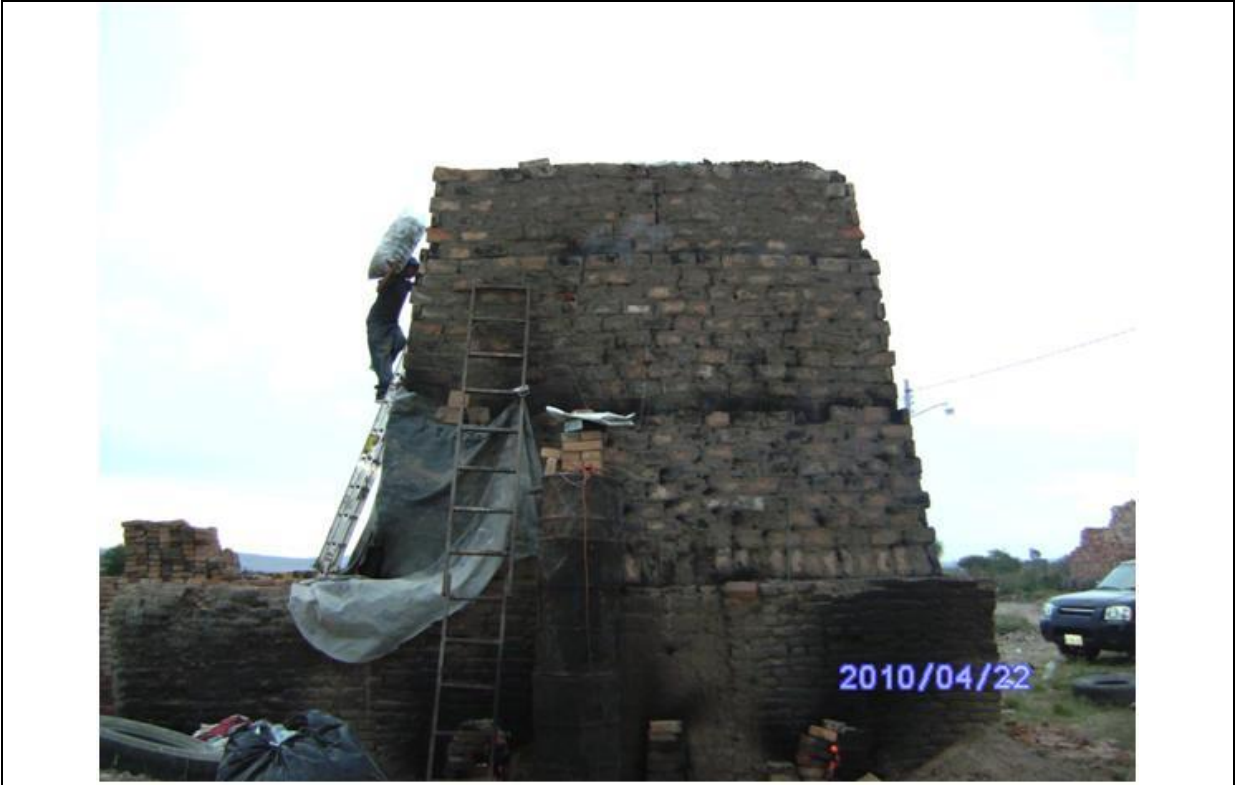
Figure 27: Detail Juventino Rosas, LP gas fired temporary kiln
