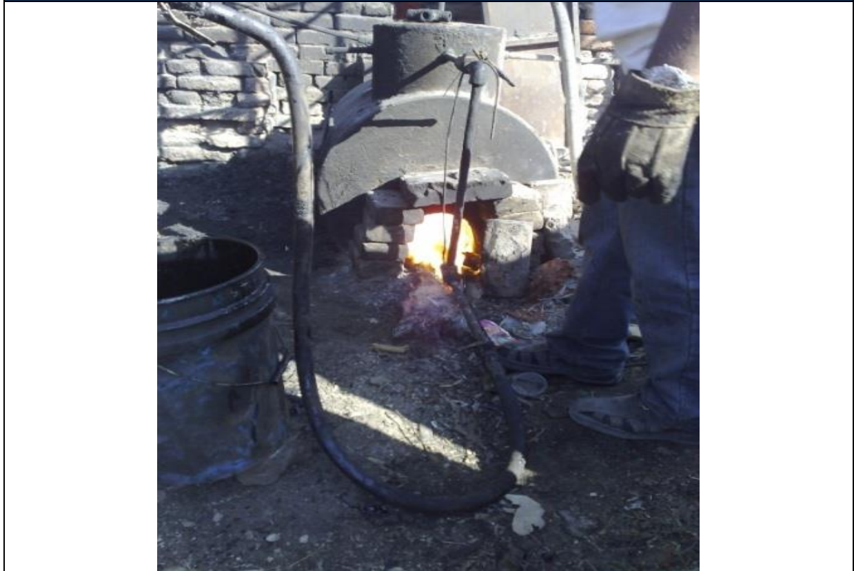
Figure 12: Detail Salamanca 1, fuel (Combustóleo) co-injection using steam
