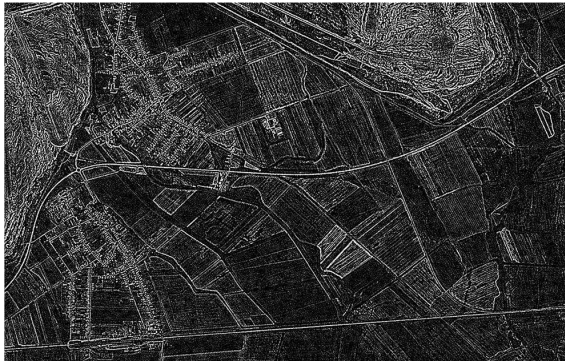
Figure 3: A standard edge extraction using the "Laplace" 3x3 kernel on the red band of Figure 2.
