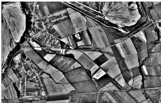
Figure 5: Contrast on larger neighbourhood using distance d=25 on the red band (25 pixel radius, ±5 Ha, in equation 1).
