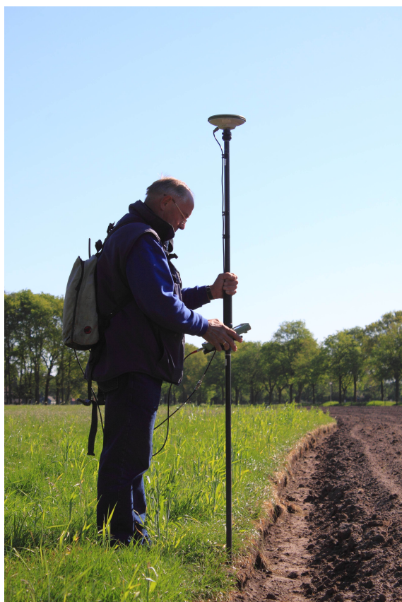
Figure 1: Surveyor measuring the agricultural parcel. Photo: courtesy of Facto Geo Meetdienst.
