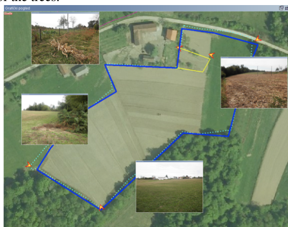
Figure 6: Green GPS points were taken using EGNOS correction, red one without it, probably due to a shadow of the trees.
