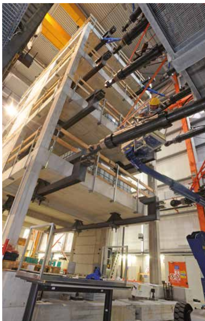
Full scale testing of a 4-storey reinforced concrete building at the JRC managed European Laboratory for Structural Assessment (ELSA).
