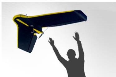
Fixed wing Sensefly (hand launched) : (copyright : www.sensefly.com )
