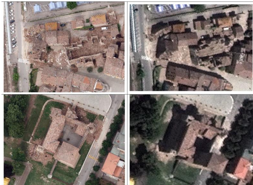
Manned Aerial platform using a Vexcel ultracam: taken under cloud canopy, with a spatial and spectral resolution superior to VHR. The original GSD was 5 cm. The image is subsampled to 20 cm. Note how the absence of shadows is actually beneficial to damage detection. (copyright : blomcgr)
