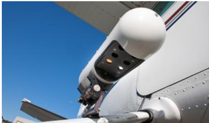
Strut mount (geovantage) on the wing of a CESSNA single engine. This system is FAA certified. (Copyright www.geovantage.com )
