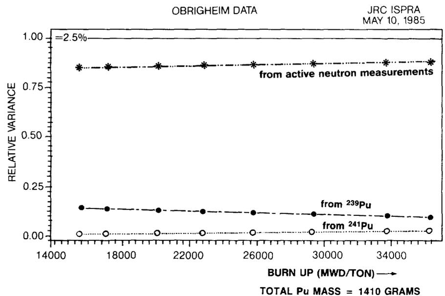
Fig. 7 - Active assay: plutonium error propagation analysis
