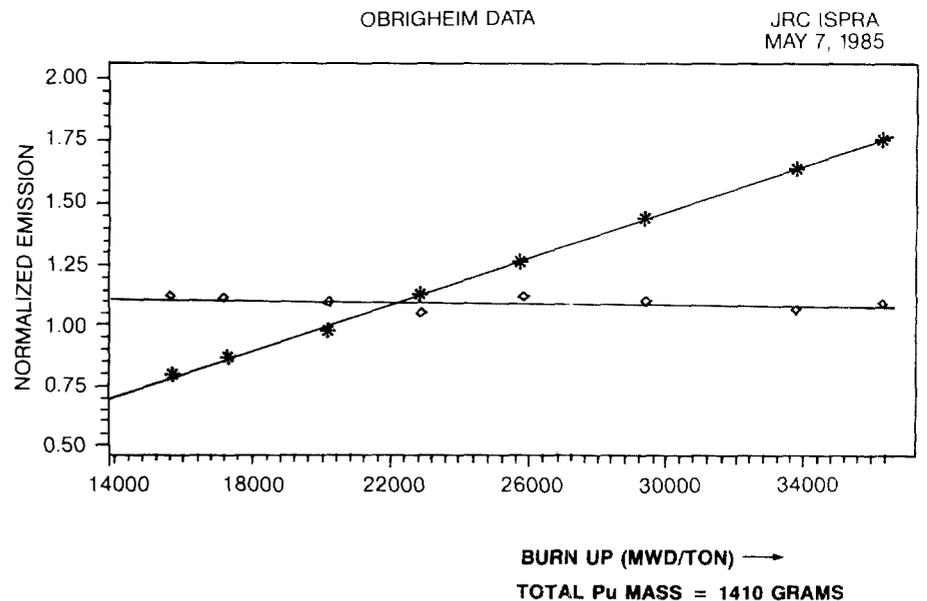
Fig. 11 - Plutonium emission analysis: normalized passive and active emissions as functions of burnup
