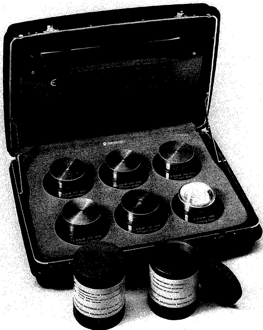
The NRM 171 / SRM 969 in its case, together with two transport containers for the single standard samples. The set is completed with an empty can, which allows comparison measurements on material with an unknown enrichment in exactly the same geometrical conditions.
