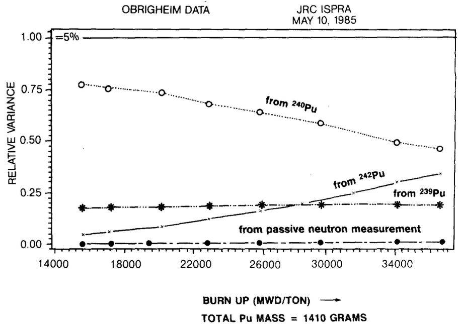
Fig. 6 - Passive assay: plutonium error propagation analysis
