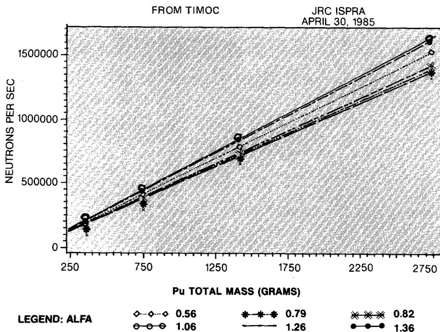
Fig. 9 - Pu active emission at different isotopic compositions vs Pu mass
