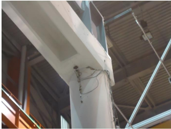
Fig. 10.19 Crack opening at the top and bottom of pier 11 after test k09
