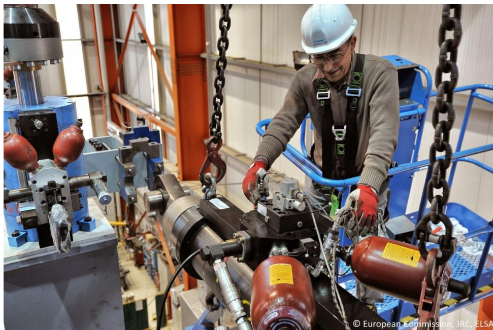
Figure A.8 Connecting hydraulic actuators at the top of piers
