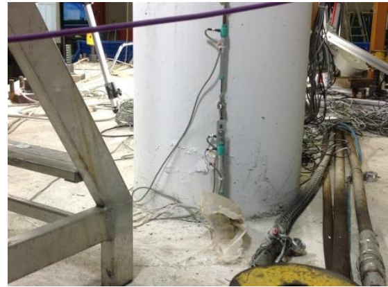
Fig. 10.19 Crack opening at the top and bottom of pier 11 after test k09
