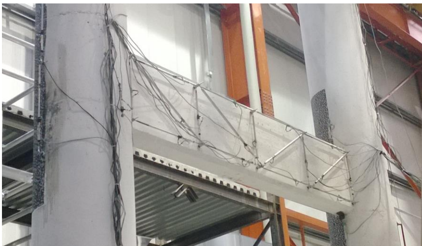
Figure 7.7 Extensimeter sensors on the transverse beam
