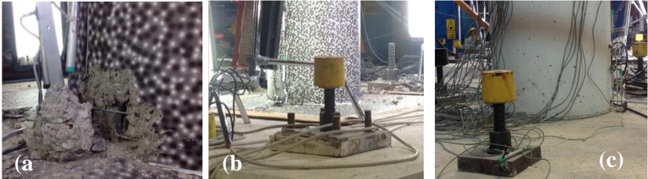
Fig. 10.30 Crack opening and buckling phenomena at the bottom section of columns in the Short (a,b) and Tall pier (c) after test k12
