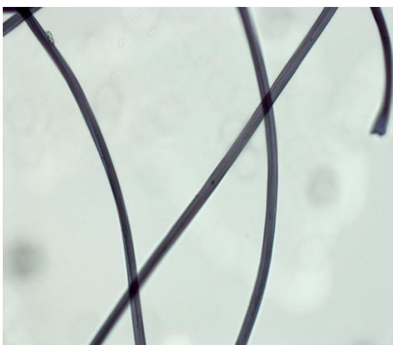
Figure 2: Microscope longitudinal analysis of sample's 304 remaining residue after applying the chemical dissolution methods 7 and 8 (28% PTT - 5% elastane - 68% modal) 200x (left) and 400x (right)
