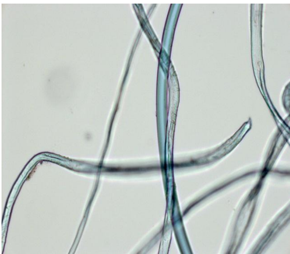
Figure 12: Microscope longitudinal analysis of sample 323 (40% PTT - 60% cotton) 200x (left) and 400x (right)
