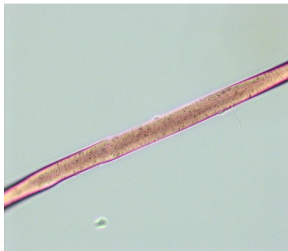
Figure 15: Microscope longitudinal analysis of the sample's 324 remaining residue after applying the chemical dissolution methods 7 and 8 (37% PTT -58% modal – 5% elastane) 200x (left) and 400x (right)
