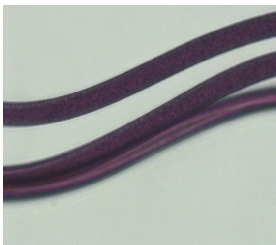
Figure 6: Microscope longitudinal analysis of sample's 306 remaining residue after applying the chemical dissolution method 4 (41% PTT - 58% polyamide) 200x (left) and 400x (right)
