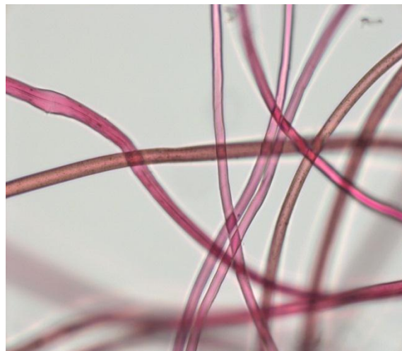
Figure 14: Microscope longitudinal analysis of sample 324 (37% PTT -58% modal – 5% elastane) 200x (left) and 400x (right)
