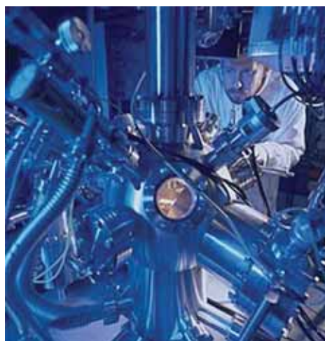
Photoemission spectrometer to study surface phenomena relevant for spent fuel corrosion processes.
