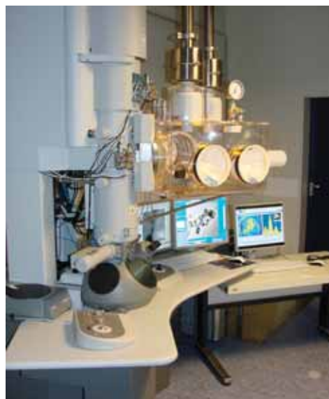
JRC transmission electron microscope facility for advanced material studies.
