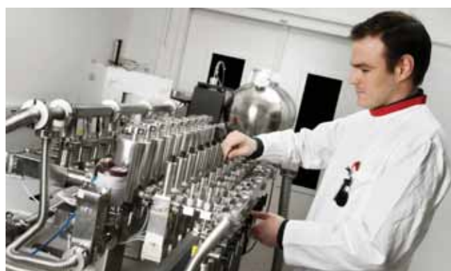
Reference measurements of \text{UF}_6 samples from enrichment plants.
