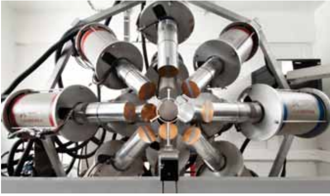
GAINS spectrometer for nuclear data measurements.
