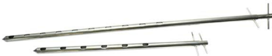
Figure 8.5: Multi-compartment sampling spear (160 cm) to sample bulk grain from various depths
