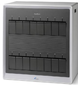
Figure 4: 'All in One' Pathogen Detection System (CEA/DRT/Leti, France). Related to Part 5.2, Genetic methods Source: http://www-leti.cea.fr
