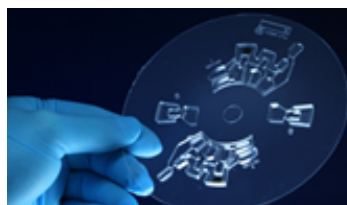
Figure 5: LabDisk and LabDisk Player prototypes, Germany Related to Part 5.2, Genetic methods Source: www.loac-hsg-imit.de
