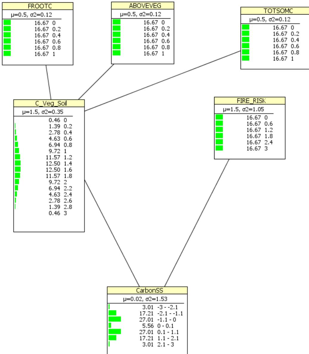
**Figure 1: Representation of the Bayesian Network to estimate stock and flow of Carbon potential. Variables are defined in Table 1. Within each monitor window, bar charts and second columns represent initial conditions of the different scores. When the network is applied to a specific area (i.e. a grid cell of forest), these conditions reflect the probability of one or more scores for that particular area.**
