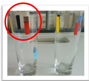
Figure 8 - Samples decoration after exposure with acetic acid 4%
