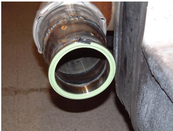
Figure 8-2 EFM Clamping: Flanges on tailpipe and exhaust flow
