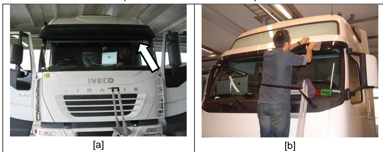
Figure 8-7 [a] Installation example for the weather station. [b] Shielding with aluminium tape
