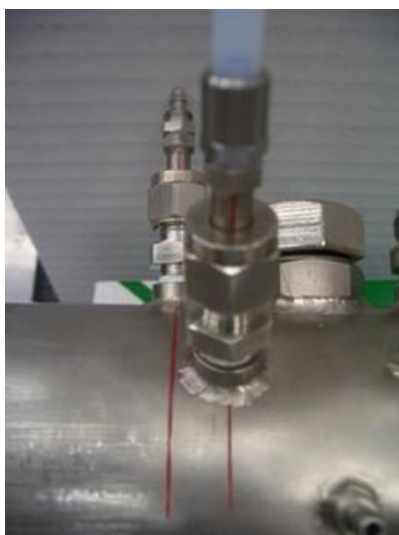
Figure 8-4 Alignment of EFM Pitot tubes
