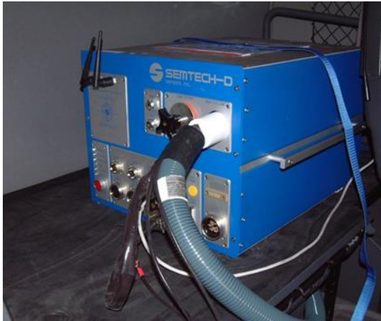
Figure 8-1 Example of secured installation of PEMS instrumentation
