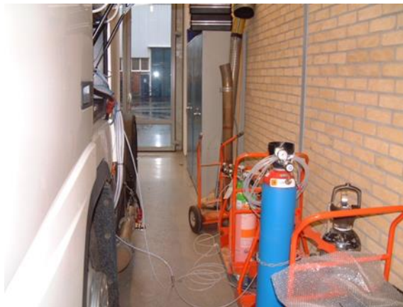
Figure 8-10 Calibration gas bottles nearby test vehicles/machines
