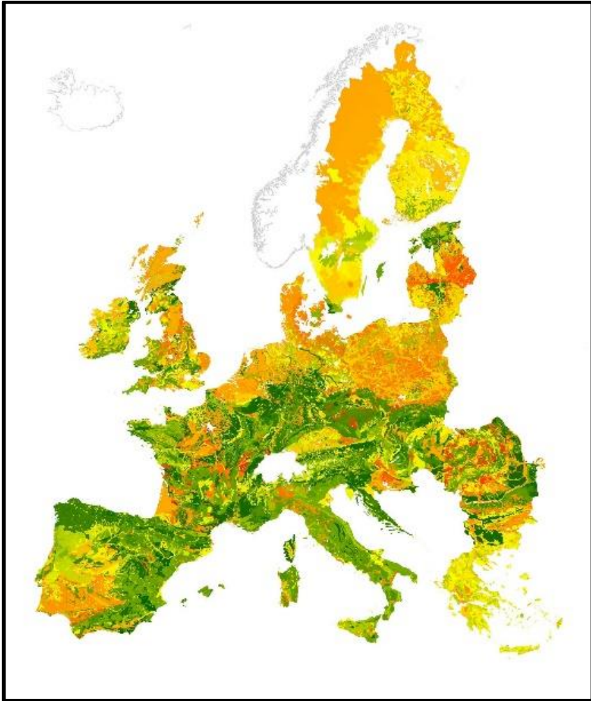
Figure 1. Predicted rates of degradation for bronze buried in soils across Europe (green = slow; yellow = fast; red = very fast)
