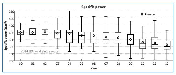
Figure 3: Boxplot representation of specific power (W/m²) for onshore wind turbines annually installed in the world. Bottom and top sides of each rectangle refers to the 25th and 75th percentiles. The horizontal line inside each rectangle represents the median and the lower and upper horizontal lines outside the rectangles are the minimum and maximum values. *Source:* JRC wind farm database.
