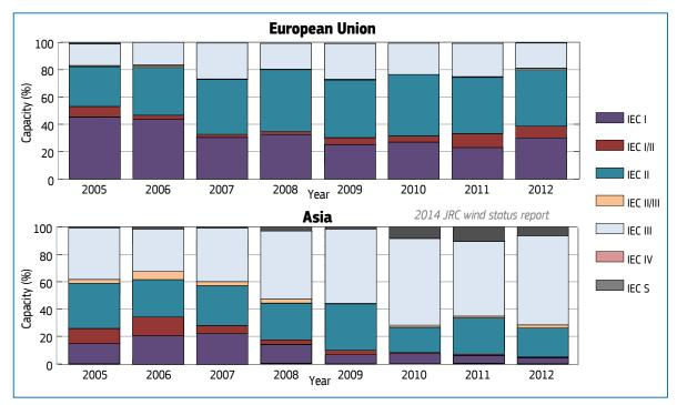
Figure 2: Evolution of the share of onshore installed capacity by wind classes (Source: JRC Database). See Table 1 for a definition of wind classes according to IEC 61400.
