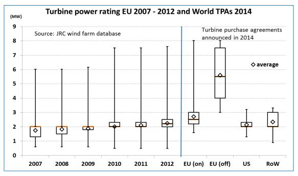
Figure 26: Turbine power rating in European onshore machines: evolution from 2007 to 2012 and comparison of data according to TPAs disclosed in 2014. *Source:* JRC database.
