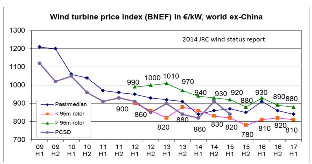
Figure 32: Evolution of wind turbine prices based on the year of delivery (past/median, less or more than 95 metres rotor) and per year of contract signature (PCSD), except China. *Source:* BNEF (2015c).
