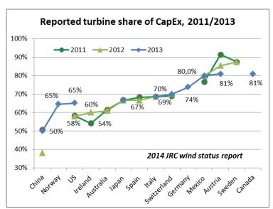
Figure 33: Turbine share of CapEx in onshore projects, 2011, 2012 and 2013. *Source:* JRC elaboration with data from IEAWind (2012, 2013, 2014).
