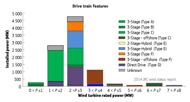
Figure 9: Drive train features classified according to wind turbine rated power. Data corresponding to installations in EU MS during 2012. *Source:* JRC Database.
