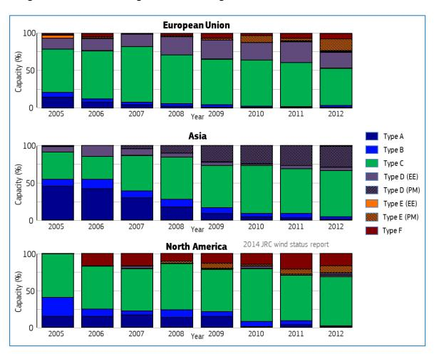
Figure 8: Evolution of the share of installed capacity by wind turbine configuration (*Source:* JRC Database). PM: permanent magnet, EE: electromagnetic excitation.
