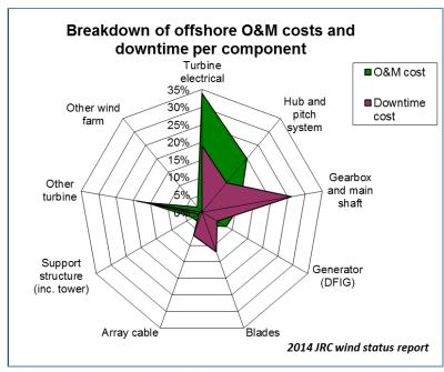
Figure 36: Breakdown of 0&M costs, in percentage of monetary units, in an offshore wind farm. *Source:* JRC elaboration from (BVG, 2012).
