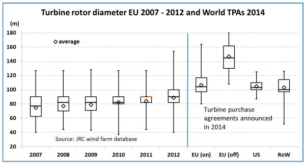
Figure 27: Rotor diameter in European turbines commissioned between 2007 and 2012, and in the TPAs disclosed in 2014. *Source:* JRC wind farm database.
