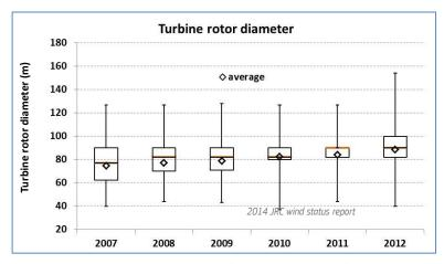
Figure 6: Boxplot representation of rotor diameters of onshore wind turbines installed each year in EU MS. (*Source:* JRC wind farm database).
