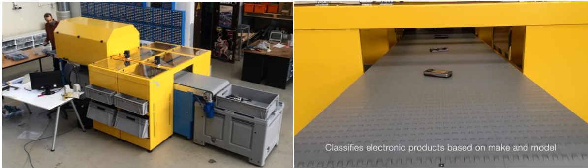
Figure 7. Pictures illustrating the e-grader at Refind technologies (Refind 2015).
