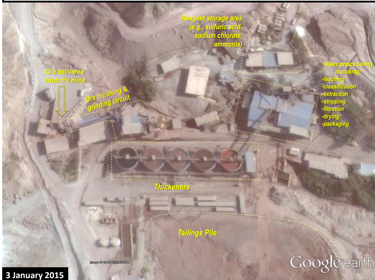
Figure 14: "Signatures" play a critical role in nuclear fuel cycle infrastructure analysis. The top view provides a flow diagram of the key components in the operation of a uranium ore concentration plant. The lower image is an operational uranium ore concentration plant, sometimes also referred to as a yellow cake production plant. Diagram source: http://www.nuclearweb.info/Uranium/Uranium_mill_news.html
