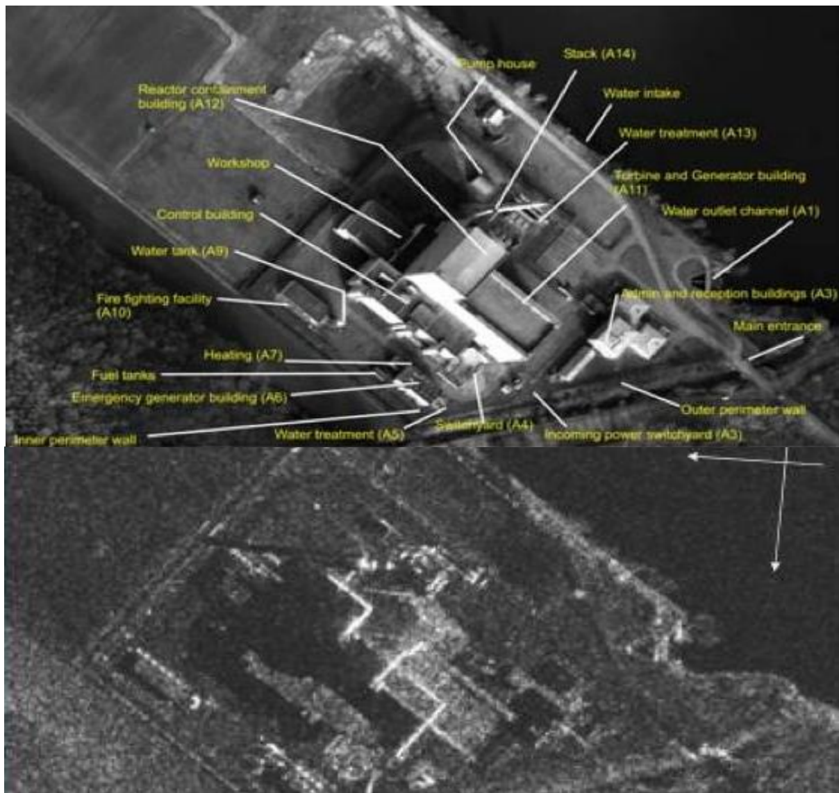
Figure 12: This figure provides an example how the comparison of electro-optical imagery (top) with radar imagery (bottom) can provide multi-sensor information synergy. Perimeter fence lines are more pronounced in the radar image. Also in the radar image, metal edges or railings on the tops of buildings create the bright reflections on the sides facing the incident radar beam (white arrow from right to left); while the opposite sides of the same structures are completely dark where the incident beam is blocked (creating discernable shadows, e.g., note the long linear shadow cast by the ventilation stack). Source: IAEA, see Reference 3.
