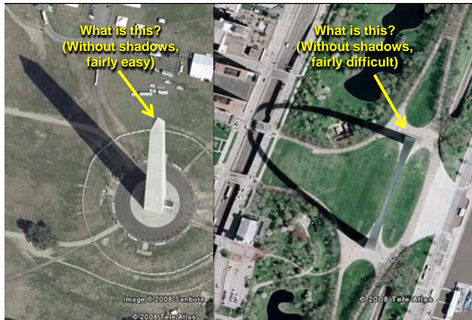
Figure 13: “Shadows” are a critical element in the analysis of commercial satellite imagery. While the oblique view of the Washington Monument makes it relatively easy to identify without shadows, the near vertical view of the St. Louis Arch would be almost impossible to identify apart from its shadow. Adapted from (a no longer active link): https://www1.nga.mil/kids/geo-int/imagery/Pages/Shadow.aspx
