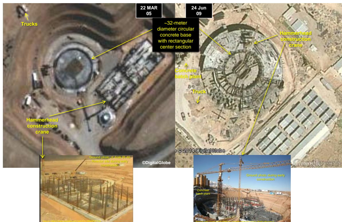
Figure 15: False Positive Exemplar, A. Left side shows the Arak, IR-40 (40 MWth), radioisotope production reactor under construction in 2005; the right side shows a large concrete structure under construction having somewhat similar attributes.
