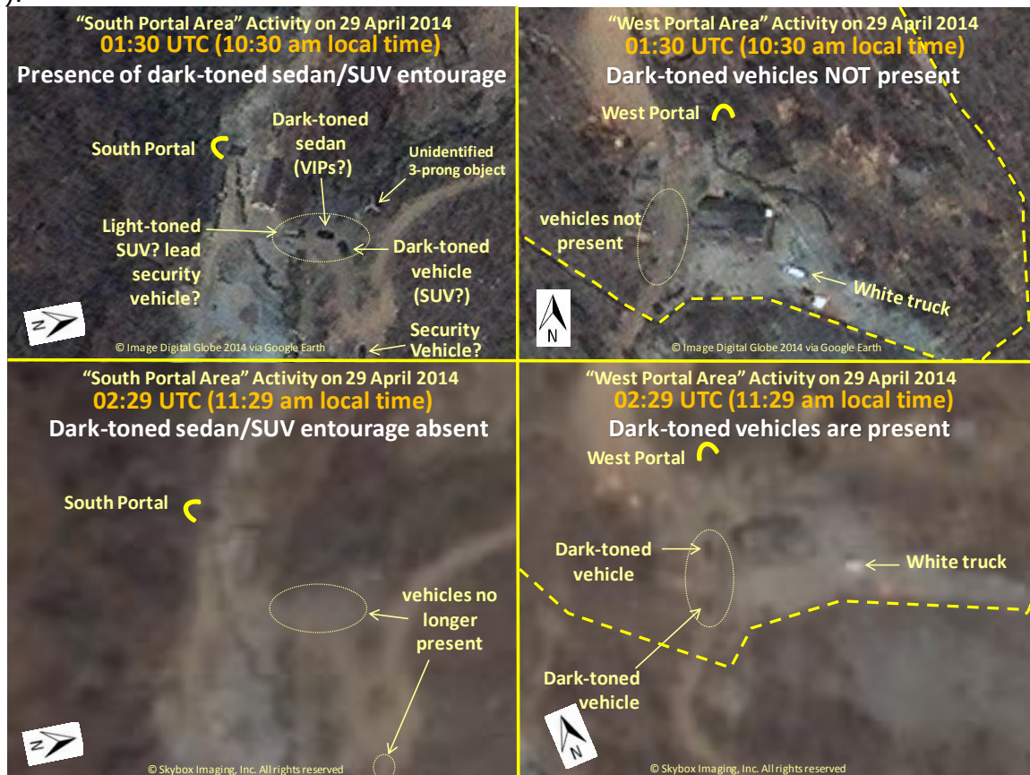
Figure 9: Multi-satellite coverage can provide synergy by allowing us to derive dark-toned vehicle movement between two nuclear test portal areas within one hour using different satellites from different vendors (left ~50 cm resolution image from DigitalGlobe, right 90 cm resolution from Skybox imaging) that is suggestive of an official visit/inspection to each of the two active test tunnels within an hour of each other.
