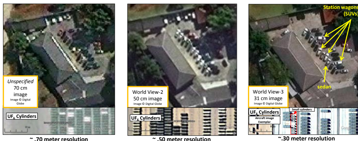
Figure 7: Interpretability comparison of high resolution commercial satellite imagery with differing resolutions below one meter. The top images are exclusively from commercial imaging satellites over Sao Paulo, Brazil; but each was acquired on a different day. 64 The bottom images are of UF 6 cylinders (lower right shows stiffening rings on large cylinders and eight small cylinders). This figure was first published in Reference 8.
