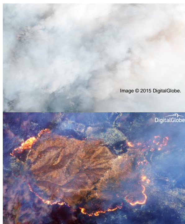
Figure 8: Short Wave Infrared (SWIR) enables viewing through the dense smoke of an active fire to the ground beneath, as well as locating the flame front and hot spots in the fire. This is a WorldView-3 image of a forest fire burning at the Happy Camp complex in California's Klamath National Forest in August 2014. The upper image is what is only discernable in the visible part of the spectrum. The smoke completely obscures the ground. The lower image is of the exact same area as viewed with SWIR imagery: the smoke disappears, and the hot spots in the fire become clearly visible. The SWIR image is a "false color" composite made from three of the eight SWIR bands (bands 6, 3, and 1) that coincidentally give an orange color to the fires.
