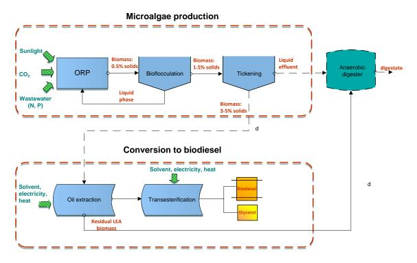
**Figure 4.1.** Main materials and energy inputs and outputs of biodiesel production from microalgae grown in ORP ("d" is the distance between the microalgal lipids production units and the conversion facilities), adapted from [14].
