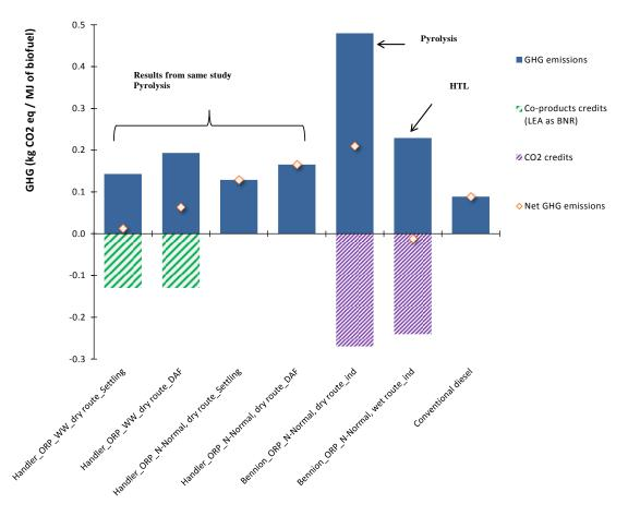
**Figure 4.7.** GHG emissions balance of 1MJ microalgal biodiesel pathways [25, 28]. The BNR displacement credits and  $CO_2$  credits are shown as negative values. Diamonds displayed on each bar represent the Net GHG emissions. For comparison, GHG emissions of WTW petroleum diesel production pathways are also indicated in the graph [131].
