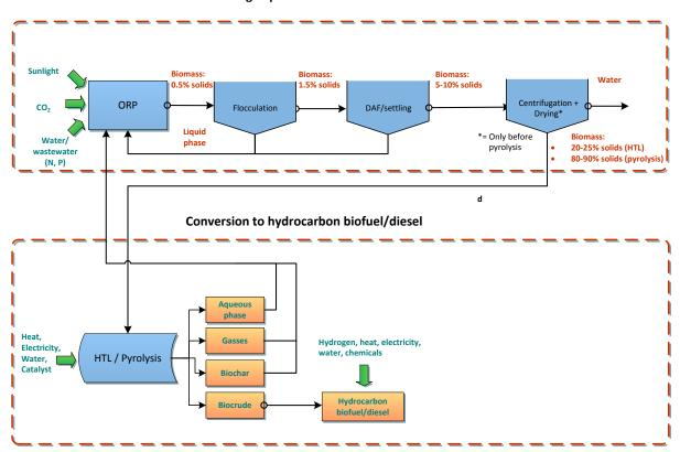
**Figure 4.5.** Main materials and energy inputs and outputs of biofuel production via pyrolysis or HTL from microalgae grown in ORP ("d" is the distance between the microalgal biomass production units and the conversion facilities), adapted from [25, 28].
