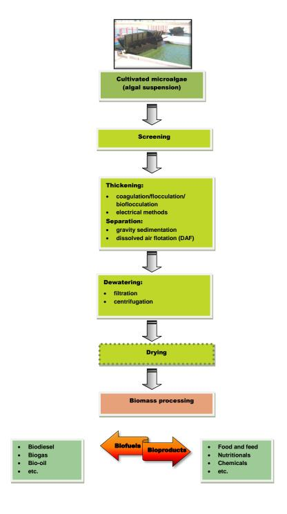
**Figure 2.11.** Process flows diagram of harvesting methods for recovery and dewatering of microalgal biomass. Drying is optional, depending on the selected downstream process for conversion of microalgae to biofuels and/or bioproducts.
