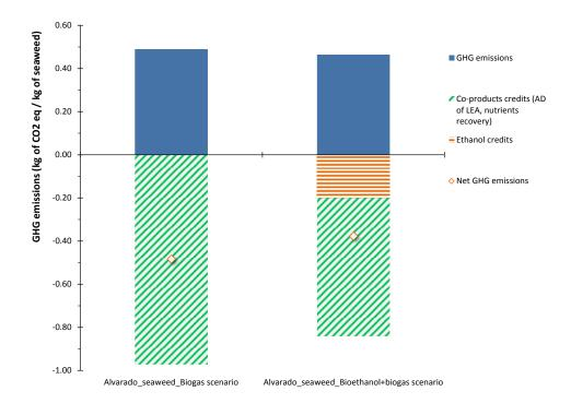
**Figure 4.10.** Total GHG emissions due to the inputs required for production of 1 kg of dry wt. seaweeds (positive values); GHG emissions offsets (negative values) due to the displacement credits given to the digestate, as well as to the ethanol and net electricity sent outside the system. The diamonds displayed on the bars represent the net GHG emissions resulting from the AD/ethanol credits considered within the biofuel pathways (GHG inputs-GHG offsets).
