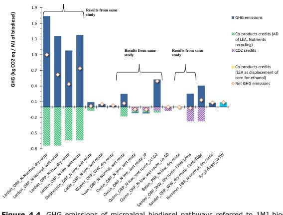
**Figure 4.4.** GHG emissions of microalgal biodiesel pathways referred to 1MJ biodiesel [24, 26, 67, 71, 72, 107]. The effects of the integration of AD of LEA biomass and displacement credits for LEA as fish feed or corn for ethanol are shown as negative values. Diamonds displayed on each bar represent the Net GHG emissions due to coproducts management. For comparison, GHG emissions of WTT and WTW petroleum diesel production pathways are also indicated in the graph [131].
