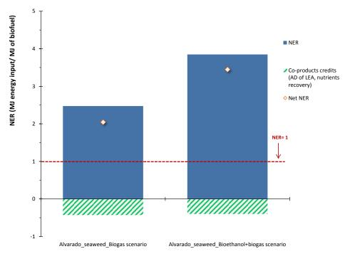
**Figure 4.9.** NER, namely the Life-cycle energy consumed/energy produced (NER <1 is desirable) for the production of biogas and/or bioethanol and biogas from seaweed via AD and fermentation in combination with AD, source: [134].
