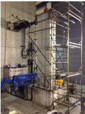
RC Pier test setup
